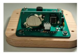
3. Plug the RTC module on the I2C interface.
